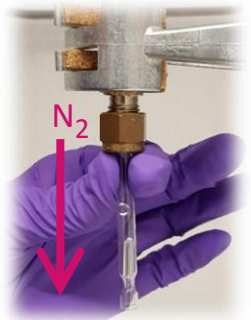
Drying in N 2 stream, alternatively by clean and lint free tissue www.gerstel.com
