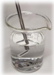
Removal of residual sample and particles by dipping into clean water
