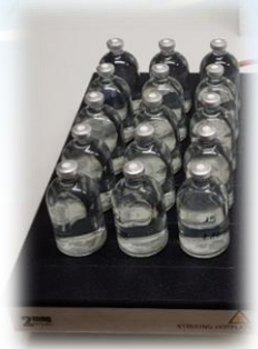
Parallel extraction – partitioning of the analytes between water and PDMS phase
