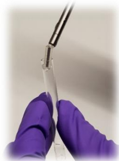
Transfer to clean TDU desorption tube
