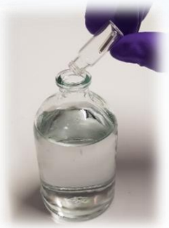
Add conditioned Twister to sample vial
