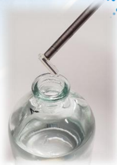
Removal of Twister after extraction
